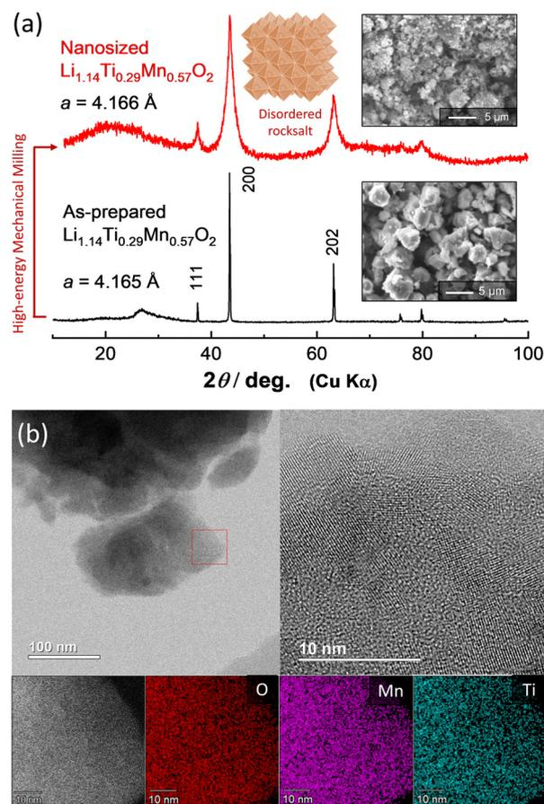
Fig. 1 (a) XRD patterns and SEM images of as-prepared and nanosized  $\text{Li}_{1.14}\text{Ti}_{0.29}\text{Mn}_{0.57}\text{O}_2$ , and a schematic illustration of disordered rock salt structure drawn using the program VESTA.<sup>27</sup> (b) STEM and EDX images of nanosized  $\text{Li}_{1.14}\text{Ti}_{0.29}\text{Mn}_{0.57}\text{O}_2$ .
