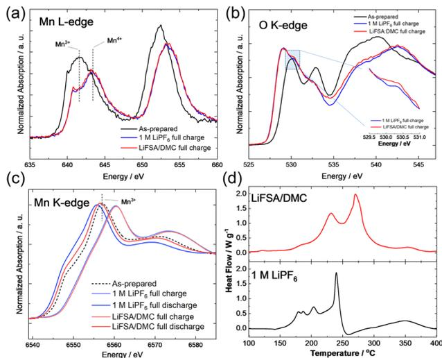
Fig. 3 (a and b) Soft and (c) hard XAS spectra of nanosized  $\text{Li}_{1.14-y}\text{Ti}_{0.29}\text{Mn}_{0.57}\text{O}_2$  on charge/discharge. (d) DSC curves of charged nanosized  $\text{Li}_{1.14-y}\text{Ti}_{0.29}\text{Mn}_{0.57}\text{O}_2$  with different electrolyte solutions.
