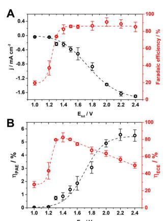
**Fig. 4** (A) Average current measured at the BDD cathode (black) and faradaic efficiency for the production of formic acid (red). (B) Energy throughput conversion efficiency for photo-assisted electrolysis ( $\eta_{PAE}$ , black), and electric-to-chemical energy conversion efficiency ( $\eta_{ECE}$ , red) as a function of  $E_{tot}$  in configuration 2. Light intensity: 25.2 mW cm<sup>-2</sup>. Lines are only a guide for the eye. The error bar shows the standard deviation (n = 3).
