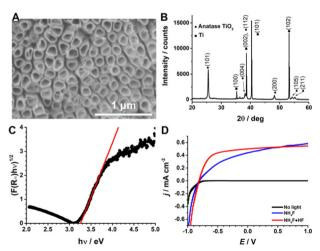
Fig. 1 Characterisation of TiO<sub>2</sub> NTs. (A) SEM micrograph, scale bar is 1 μm. (B) XRD spectrum. (C) Kubelka-Munk plot. (D) Photoelectrochemical response measured by cyclic voltammetry at 100 mV  $\rm s^{-1}$  in 0.5 M KOH with light applied of 6.5 mW cm<sup>-2</sup>, for TiO<sub>2</sub> NTs fabricated with addition of NH<sub>4</sub>F (blue) or NH<sub>4</sub>F·HF (red and black). Reference electrode: Ag/AgCl, KCl
