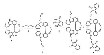
Scheme 1 Synthetic pathway leading to chiral emitters 3 and 4. Reaction conditions: (i) 1,3-dibromopropane, NaH, DMF, rt, 89%; (ii) KOtBu, NMP, 60 °C, 42 and 51% for 3 and 4, respectively. Further details are reported in the ESI.†
