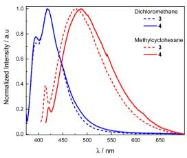
Fig. 3 Normalized luminescence spectra in dichloromethane (blue) and methylcyclohexane (red) of **3** (dotted lines) and **4** (solid lines) ([c]  $\sim 10^{-5}$  M)
