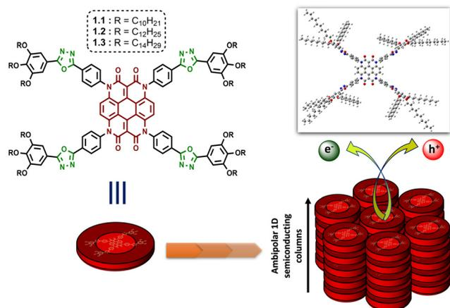
Fig. 1 Molecular structure of oxadiazole integrated heterocoronene-based columnar DLCs for ambipolar charge transport (optimized geometry of **1.1** is shown in top-right corner).
