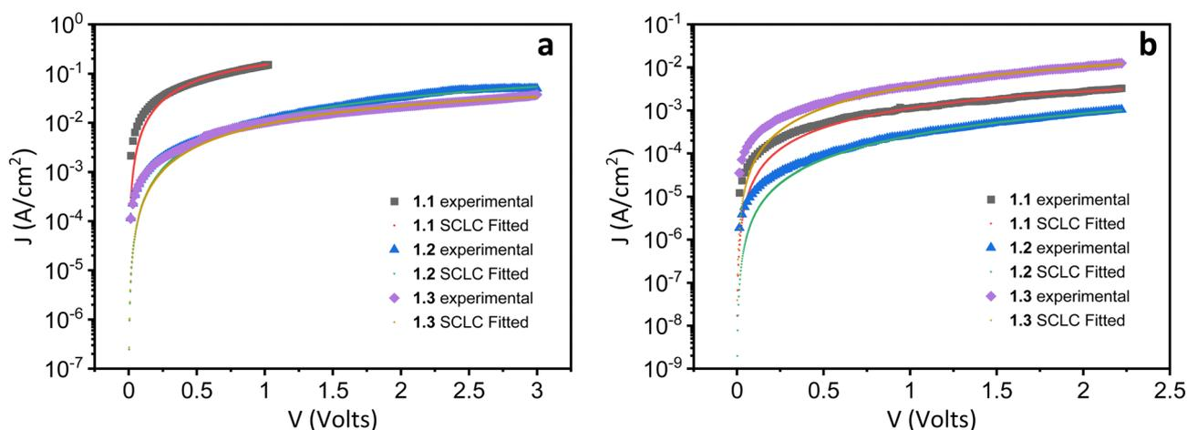
Fig. 3 Current density–voltage characteristics as a semi-log plot obtained for (a) hole and (b) electron mobilities extracted from SCLC devices in the thin film of compounds **1.1–1.3** at room temperature.
