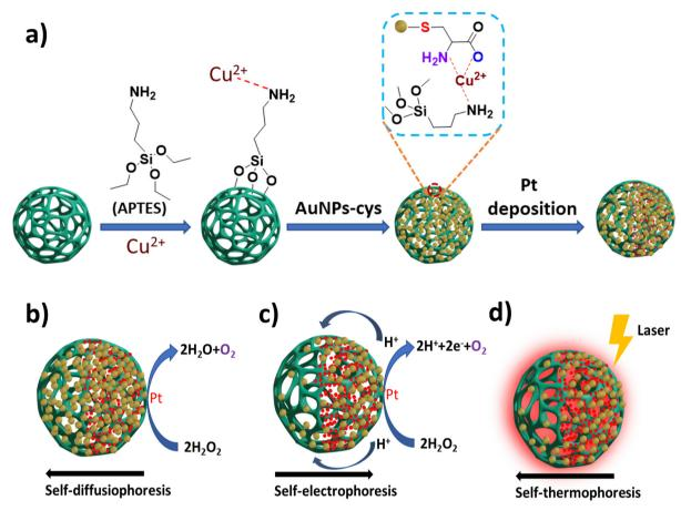
Fig. 7 (a) Schematic representation of the synthesis of core@satellite JMPA nanomotors. (b-d) Schemes representing self-diffusiophoresis, selfelectrophoresis and self-thermophoresis mechanisms of JMPA nanomotors. Information adapted from ref. 66.
