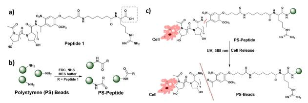
Fig. 12 (a) Peptide 1 structure. (b) Schematic representation of the reaction of aminated PS beads with the carboxylic acid group (circled in Fig. 12a) by the EDC-NHS coupling reaction. (c) Cell captured by phototaxis and release of beads from cells under UV, 365 nm. Information adapted from ref. 102.
