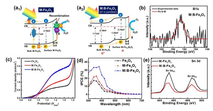
Fig. 10 (a) Schematic illustration of an energy band diagram and charge transfer process of (a<sub>1</sub>) M-Fe<sub>2</sub>O<sub>3</sub> and (a<sub>2</sub>) M:B-Fe<sub>2</sub>O<sub>3</sub>, (b) XPS B 1s spectra, (c) J-V curves, (d) IPCE, and (e) XPS Sn 3d spectra. Reproduced from ref. 44 with permission from American Chemical Society, Copyright 2018.
