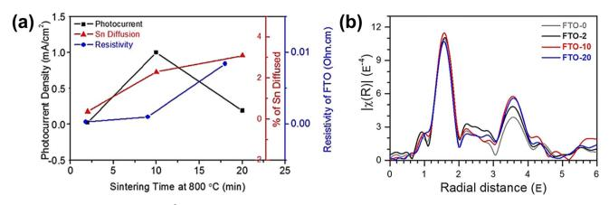
Fig. 8 (a) Photocurrent density (mA cm $^{-2}$ ), atomic percent of Sn diffusion of hematite photoanodes, and resistivity of the FTO substrate sintered at 800 °C for 2, 10, and 20 min.  $k^3$ -weighted Fourier transforms for (b) Sn K-edge EXAFS of FTO substrates sintered at 800 °C for 0, 2, 10, and 20 min. Reproduced from ref. 62 with permission from American Chemical Society, Copyright 2015.
