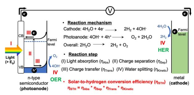
Fig. 1 Schematic illustration of the basic principle of the PEC water splitting system.
