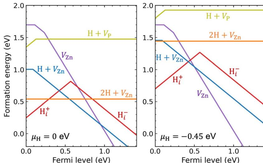
Fig. 4 Formation energies as a function of Fermi level for hydrogen interstitial ( $H_i$ ) and hydrogen-vacancy complexes, including the  $H + V_{Zn}$ ,  $2H + V_{Zn}$ , and  $H + V_P$ , in  $Zn_3P_2$ , under Zn-poor/P-rich condition and at two different chemical potentials of H ( $\mu_H$ ): the H-rich limit  $\mu_H = 0$  eV (left panel) and a lower  $\mu_H$  at  $-0.45$  eV (right panel). For comparison the formation energy of  $V_{Zn}$  is also depicted.
