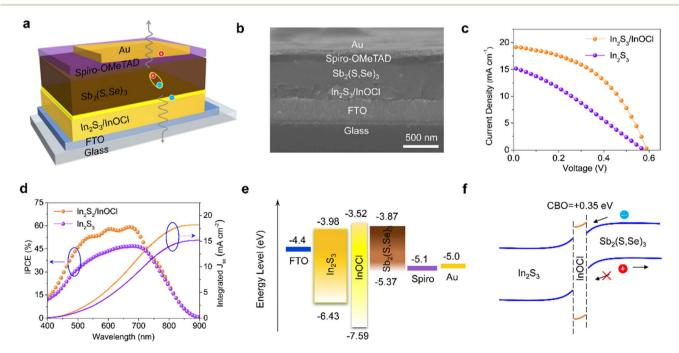
Fig. 4 (a and b) The schematic illustration and cross-sectional SEM image of a complete device with the configuration of FTO/In<sub>2</sub>S<sub>3</sub>/InOCI/  $Sb_2(S,Se)_3/spiro-OMeTAD/Au$ , (c) J-V and (d) IPCE curves of the best-performing devices based on  $In_2S_3$  and  $In_2S_3/InOCl$  buffer layers, (e) energy level diagrams of functional layers of  $Sb_2(S,Se)_3$  solar cells, and (f) diagram of energy band alignments at the  $In_2S_3/InOCI/Sb_2(S,Se)_3$  interface.
