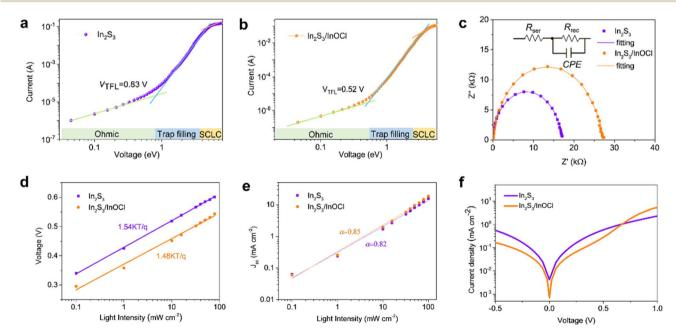
Fig. 5 (a and b) The SCLC measurements of  $\ln_2S_3$  and  $\ln_2S_3/\ln OCl$ -based electron-only single-carrier devices, and (c) the impedance spectroscopy spectra, (d) light intensity-dependent  $V_{oc}$  measurements, (e) light intensity-dependent  $J_{sc}$  measurements, and (f) dark J-V curves of  $\ln_2S_3/\ln OCl$ -based Sb<sub>2</sub>(S,Se)<sub>3</sub> solar cells.
