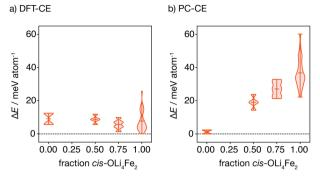
Fig. 4 Distributions of structural energies for all  $2 \times 2 \times 2$  structures consisting solely of OLi<sub>4</sub>Fe<sub>2</sub> oxygen coordination environments, calculated using (a) the DFT-CE DFT-fitted cluster expansion model, and (b) the PC-CE point-charge model. For each model, the distributions are subdivided according to the fraction of cis- versus trans-OLi<sub>4</sub>Fe<sub>2</sub> octahedra in each structure.
