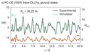
Comparison of pair-distribution functions (PDFs) obtained from X-ray total scattering and simulated PDF data for Li<sub>2</sub>FeSO for structural models generated for (a) the DFT-fitted cluster-expansion model (DFT-CE), (b) the RANDOM model, and (c) the PC-CE point-charge model
