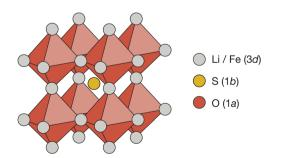
Fig. 1 The reported antiperovskite structure (space group  $Pm\bar{3}m$ ) of Li<sub>2</sub>FeSO.<sup>24</sup> Oxygen occupies the 6-coordinate octahedral Wyckoff 1a site. Sulfur occupies the 12-coordinate Wyckoff 1a site. Lithium and iron are distributed over the Wyckoff 3d sites in a 2:1 ratio.
