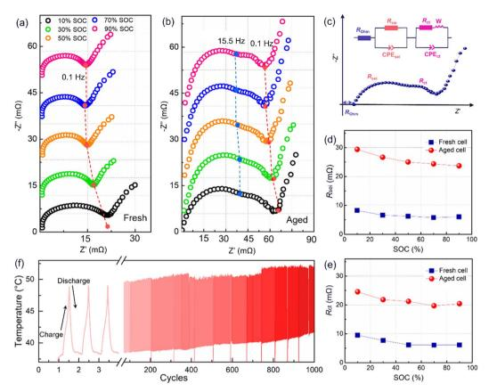
Fig. 2 EIS spectra at different SOCs for a (a) fresh cell and (b) an aged cell; (c) schematic illustration and an equivalent circuit used to fit the EIS Nyquist plots; the fitted results for (d)  $R_{\text{sei}}$ , and (e)  $R_{\text{ct}}$ ; (f) the temperature tested using a temperature sensing probe on the outer surface of the cell.
