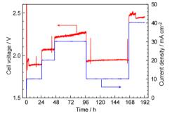
Fig. 4 Cell voltage and current density as a function of the elapsed time in the measurements for Fig. 3. The operating temperature was 120 °C and the cell was operated in a constant current mode.
