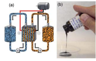
Fig. 6 (a) Schematic diagram of a SSFB and (b) picture of typical electroactive paste. Reprinted with permission from ref. 47, copyright 2011. Wilev.
