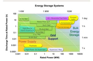
Fig. 3 Energy storage technologies as a function of their nominal power and discharge time. Mechanical (yellow), magnetic (light grey) thermal (orange) chemical (purple), electrochemical (green) and electrophysical (blue-green).
