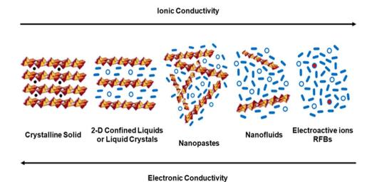
Fig. 7 Schematic comparative diagram of the stages involved in moving from compact solid electrode materials to dilute nanofluids and RFB solutions.
