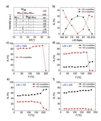
Fig. 4 (a) PXRD patterns of HC- and SC-PLA microspheres. (b) The relative degree of crystallinity  $(X_c)$  of the HC and SC crystallites. (c-f)Relative degree of  $X_c$  versus temperature in the range of 25 to 220 °C for HC and SC crystallites of PLA with L/D ratios of 10/0 (c), 9/1 (d), 7/3 (e), and 5/5 (f).
