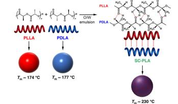
**Fig. 1** Schematic illustration of the fabrication of microspheres from HC- and SC-PLA by the O/W miniemulsion method.
