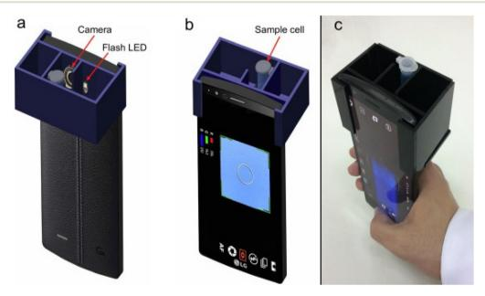
Fig. 2 (a-c) show the portable handheld RGB-based colorimetry device for the self-referenced solution-based determination of the water content in ethanol [this figure has been reproduced from ref. 40 with permission from Elsevier Sciences, copyright 2020].
