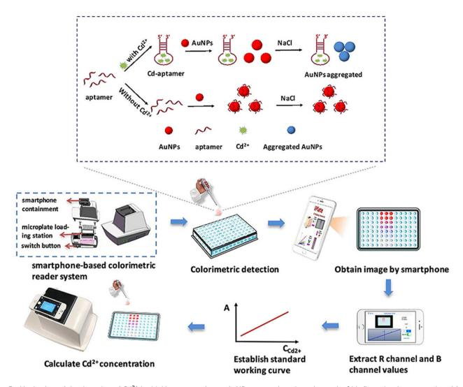
Fig. 5 Mechanism of the detection of Cd<sup>2+</sup> in drinking water using an AuNP-aptamer based sensing probe [this figure has been reproduced from ref. 56 with permission from Elsevier Sciences, copyright 2020].
