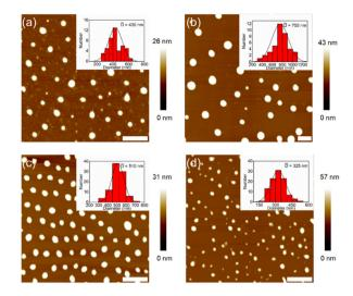
Fig. 2 Morphologies of the assemblies from DSPs. AFM images on mica from aqueous solutions of SP-GA-MeG1 (a), SP-GA-EtG1 (b), SP-AG-MeG1 (c) and MeG1-GA-SP (d). C = 0.15 mg mL<sup>-1</sup>, scale bar = 2 µm.
