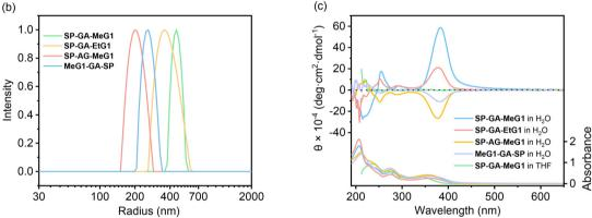
Fig. 1 Assembly of DSPs in various solvents at 10 °C. (a)  $^{1}$ H NMR spectra of SP-GA-MeG1 in a mixture of D<sub>2</sub>O/THF- $d_8$  at 10 °C with different volume fractions of water,  $f_w$ . C = 1.0 mg mL $^{-1}$ . (b) DLS results of DSPs in aqueous solutions. C = 0.15 mg mL $^{-1}$ . (c) CD spectra of DSPs in different solvents. C = 0.3 mg mL $^{-1}$ .
