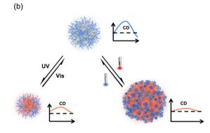
Chart 1 Illustration of supramolecular assembly of the dendronized spiropyrans (DSPs) (a) in aqueous solutions into chiral spheres with chiralities dually tunable by irradiation and temperature (b).
