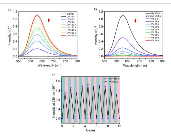
Fig. 4 Fluorescence spectra of SP-GA-MeG1 aqueous solutions after irradiation with UV (a) and visible light (b), and its fluorescence intensity at 630 nm after alternate irradiation with UV and visible light (c).  $\lambda_{\rm ex}$  = 535 nm,  $\lambda_{\rm UV}$  = 254 nm,  $\lambda_{\rm Vis}$  > 450 nm, T = 10 °C, C = 0.15 mg mL<sup>-1</sup>.
