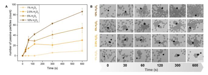
Fig. 3 (A) Quantification of rafting behavior with  $SiO_2$  colloids and (B) optical microscopy snapshots after different time intervals at different  $H_2O_2$  concentrations. A UV light of intensity 19.08 W cm<sup>-2</sup> and wavelength 385 nm is used.
