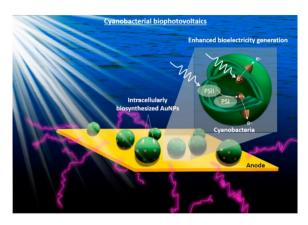
Fig. 8 Conceptual image of the proposed work on the cyanobacterial biophotovoltaics for enhanced biophotoelectricity generation. Intracellularly biosynthesized Au NPs will improve cyanobacterial electron harvesting and extracellular electron transfer. Reproduced from ref. 172 with permission from Elsevier, Copyright 2021.
