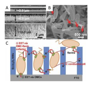
**Fig. 3** (A) Cross-section SEM images of the flat FTO film and SINW/FTO with the nanowire lengths of 2.47, 5.80, and 9.85  $\mu$ m. (B) SEM images of SINW/FTO electrodes integrated with microbes of *S. loihica* PV-4 after 25 h electrochemical culture at 0.2 V. The red arrows mark the pili grown among cells. (C) Cartoon illustrating the active EET pathways on the SiNW/FTO electrode. Reproduced from ref. 133 with permission from Wiley Online Library, Copyright 2018.
