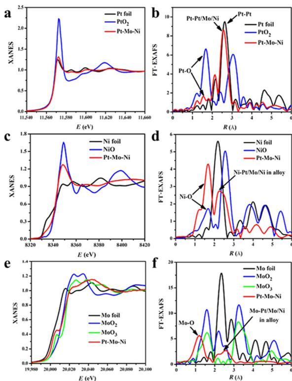
**Fig. 2** XAS analyses of the PtMoNi NWs. XANES (a) and EXAFS (b) analysis of Pt  $L_{3}$ -edge (FT range, 4.3 to 14.5  $\text{\AA}^{-1}$ ). XANES (c) and EXAFS (d) analysis of Ni K-edge (FT range, 2.5 to 12.5  $\text{\AA}^{-1}$ ). XANES (e) and EXAFS (f) analysis of Mo K-edge (FT range, 2.0 to 10.5  $\text{\AA}^{-1}$ ). Reprinted with permission from ref. 51. Copyright 2017 from AAAS.
