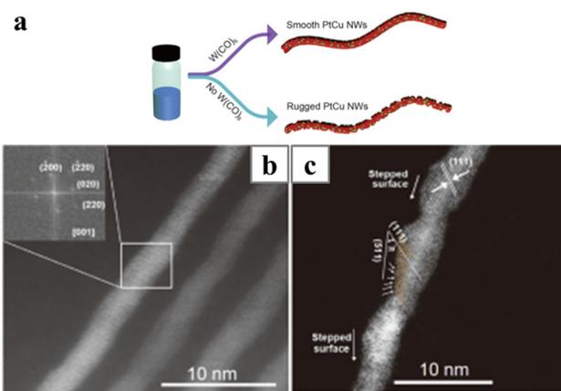
**Fig. 7** (a) Schematics illustrating the effect on the W(CO)<sub>6</sub> on the surface of the PtCu nanowires and (b and c) HAADF-STEM images of (b) the smooth PtCu nanowires (inset showing the corresponding FFT pattern) and (c) the rugged PtCu nanowires. Reprinted with permission from ref. 82. Copyright 2020 from Springer Nature.
