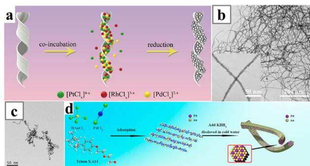
**Fig. 24** (a) Schematics illustrating the formation of PtRhPd nanocoils and (b) TEM image of the PtRhPd nanocoils. (c) TEM image of AuPd nanowires synthesized with Triton X-114 as the structure-directing reagent and (d) the schematics illustrating the formation mechanism of the Triton X-114 induced synthesis. Reprinted with permission from ref. 181 and 182. Copyright 2020 from the American Chemical Society and 2020 from Elsevier.
