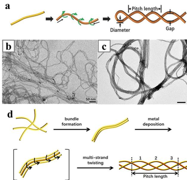
**Fig. 20** (a) Schematics illustrating the twisting of Au–Ag double helix nanowires. (b) TEM image of ultrathin Au–Ag alloy helices. (c) TEM image of AuPd nanoropes. (d) Schematics illustrating the braiding of AuPd nanoropes. Reprinted with permission from ref. 156 and 157. Copyright 2018 from WILEY-VCH GmbH and 2020 from the American Chemical Society.
