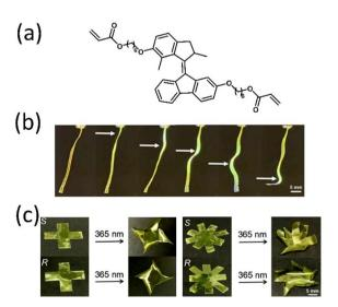
Fig. 21 (a) Molecular structure of a rotary motor. Light-powered (b) wavy motion and (c) helical motion of the motorized LC film (scale bar is 5.0 mm). Reproduced with permission.<sup>200</sup> Copyright 2022, The Authors, published by American Chemical Society.
