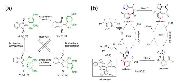
Fig. 3 (a) Molecular structures of hemithioindigo motor with four stable diastereoisomers and their cyclic motion. The "rotors" are colored green.<sup>76</sup> (b) Structure and mechanism of directional rotation in the chemically-fueled motor.<sup>80</sup>
