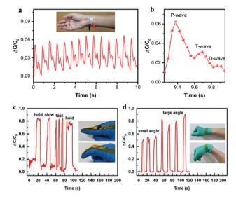
Fig. 5 The main application of capacitive sensors, (a) and (b) are pulse wave monitoring:141 (c) and (d) are finger and wrist bending.142 Reproduced with permission. Figure (a and b) has been adapted/ reproduced from ref. 141 with permission from American Chemical Society, copyright 2020. Figure (c and d) has been adapted/reproduced from ref. 142 with permission from Wiley-VCH GmbH, copyright 2021.
