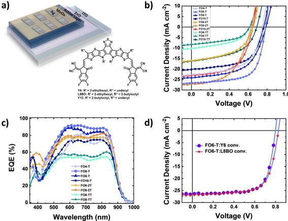
Fig. 2 (a) Device architecture of the solar cells (inverted structure) and molecular structure of the NFAs, (b) J-V curves of devices under AM1.5G illumination, (c) EQE spectra of the OPV devices and (d) J-V curves for devices with conventional structure L8BO and Y6 as acceptors under AM1.5G illumination.
