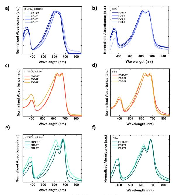
Fig. 1 UV-vis absorption spectra of polymers in solution in CHCl<sub>3</sub> (a) FOR-T polymers, (c) FOR-2T polymers, and (e) FOR-TT polymers, and in thin film (b) FOR-T polymers, (d) FOR-2T polymers and (f) FOR-TT polymers. The solutions were prepared at a 5  $\mu$ M concentration and thin films were prepared from a 10 mg mL<sup>-1</sup> solution and spin coated on glass slides.
