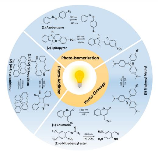
Fig. 2 Schematic illustration of photo-reactions that were utilized in designing photo-responsive hydrogels.
