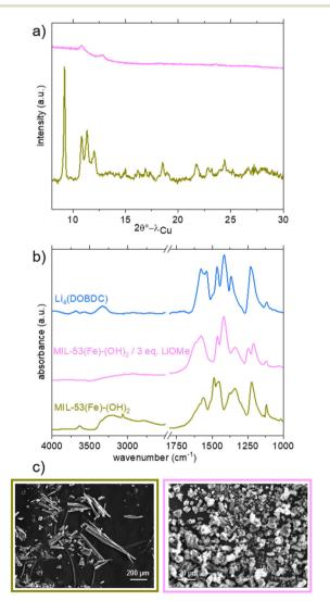
Fig. 5 Characterisation of MIL-53(Fe)-(OH)<sub>2</sub> and its lithiated product from LiOMe in MeOH/THF. a) PXRD patterns ( $\lambda$  = 1.5406 Å); b) IR spectra; c) SEM pictures. Data related to dry MIL-53(Fe)-(OH)2, Li<sub>4</sub>(DOBDC) and the lithiation product are shown in khaki, blue and pink, respectively.
