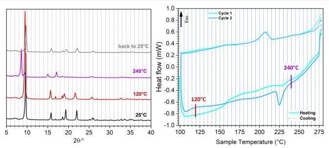
Fig. 3 VT-XRPD patterns of F<sub>4</sub>-MIL-53(Al) at room temperature (25 °C – black), before the phase transition (120 °C red), after the phase transition (240 °C purple) and after returning to the room temperature (25 °C - light grey) (left). DSC profile of F<sub>4</sub>-MIL-53(Al) (right): first cycle (cyan) and second cycle (light blue). Full and dotted curves refer to the heating and cooling cycles respectively (right).
