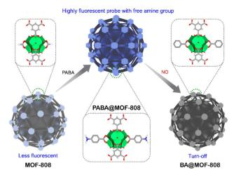
Scheme 1 Schematic illustration of post engineering of a chemically stable MOF and further detection of nitric oxide (NO) with a free amine group containing florescent probe (PABA@MOF-808).
