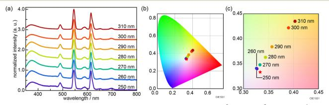
Fig. 3 (a) Emission spectra and (b) CIE chromaticity diagram of MIL-103(Eu<sub>x</sub>Gd<sub>y</sub>Tb<sub>z</sub>; Eu =  $8.3 \times 10^{-5}$ , Tb =  $8.1 \times 10^{-3}$ , Gd =  $9.92 \times 10^{-1}$ ) at various excitation wavelengths. (c) Enlarged view of Fig. 3b.
