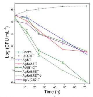
Fig. 6 Colony growth curves (CFU  ${\rm mL}^{-1}$ ) of *P. roqueforti* at different incubation times, using Ag/UiO-66 solids.
