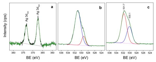
Fig. 9 XPS spectra: a) Ag 3d region in the Ag/U(0.75)T sample; b) O 1s region in UiO-66; c) O 1s region in the Ag/U(0.75)T sample.
