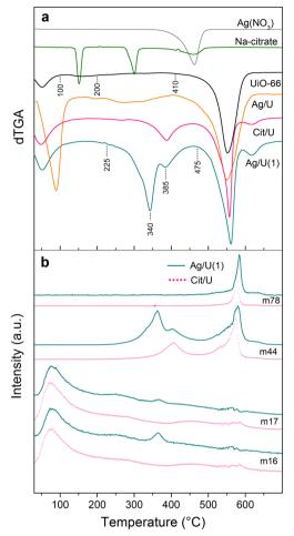
Fig. 2 a) TGA derivative profiles (dTGA); b) TGA-MS for Aq/U(1) (solid line) and Cit/U (dotted line). Note: m16 (O2, H2O); m17 (OH, H2O); m44 (CO<sub>2</sub>); m78 (C<sub>6</sub>H<sub>6</sub>).
