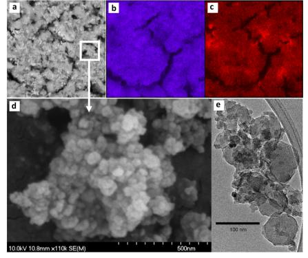
Fig. 7 SEM micrographs of Ag/U(0.75)T sample: a) SEM image of a wide region of the solid; b) mapping of silver by EDS in the selected region; c) mapping of zirconium by EDS in the selected region; d) high magnification image by FE-SEM; e) TEM image.
