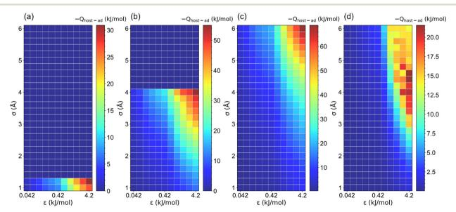
Fig. 8 The host-adsorbate interaction ( $Q_{host-ad}$ ) between pseudo material and ethanol under various LJ parameters ( $\sigma$  and  $\varepsilon$ ) for (a) l=5, (b) l=7.5, (c) l=10 and (d) l=35 Å structures.
