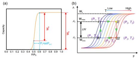
Fig. 2 Schematic (a) adsorption isotherm and (b) thermodynamic cycle of adsorption heat pumps; the blue and red curves represent the lowtemperature and high-temperature adsorption isotherms, respectively, where A is the adsorption potential.
