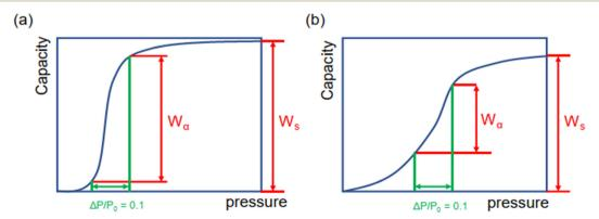
Fig. 3 Schematics of stepwise adsorption isotherms with (a) large and (b) small  $W_{\alpha}/W_{s}$ .
