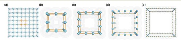
Fig. 1 The schematic figure of (a) the supercell of simple cubic crystal and cubic crystal of pseudo materials with l = (b) 5, (c) 7.5, (d) 10 and (e) 35 Å.
