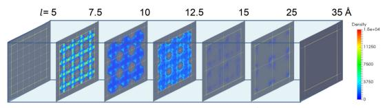
Fig. 10 The ethanol adsorption density distribution of  $W_s$  with fixed  $\sigma = 3$  Å,  $\varepsilon = 4.2$  kJ mol<sup>-1</sup> for l = 5 Å (6 × 6 × 6), 7.5 Å (4 × 4 × 4), 10 Å (3 × 3 × 3), 12.5 Å (3 × 3 × 3), 15 Å (2 × 2 × 2), 25 Å (2 × 2 × 2) and 35 Å (1 × 1 × 1) structures.
