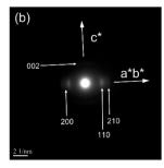
Fig. 5 (a) TEM image and (b) selected area electron diffraction patterns of PTh from 1.
