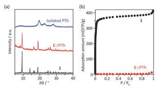
Fig. 3 (a) XRPD patterns of  $\mathbf{1}$ ,  $\mathbf{1} \supset PTh$ , and PTh liberated from  $\mathbf{1}$ . (b)  $N_2$  adsorption isotherms of 1 and 1  $\supset$  PTh at 77 K (1;  $S_{BET}$  = 1447  $m^2 g^{-1}$ , 1  $\supset$  PTh;  $S_{BET} = 4 m^2 g^{-1}$ ).
