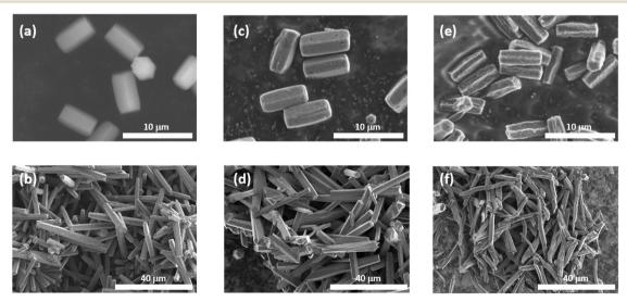
Fig. 4 SEM images of (a and b) 1 with different lengths obtained by the coordination modulation method, (c and d) 1  $\supset$  PTh, and (e and f) PTh isolated from 1. The morphologies and size of the recovered PTh objects retained those of the original hosts.
