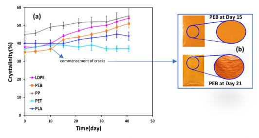
Fig. 2 Crystallinity of selected plastics during accelerated weathering (a) and photos showing PEB after days 15 and 21 (b). DSC parameters are expressed as average quantities  $\pm$  standard deviations from analysing three different subsamples for each sample (n=3).
