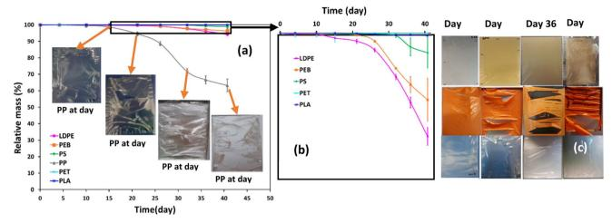
Fig. 1 Temporal mass loss for six selected polymers during accelerated weathering. Average quantities ± standard deviations were obtained by weighing each sample three times 24 h after removal from the weathering chamber (n = 3). The photos in (a) show PP at selected time intervals, while (b) magnifies data for all polymers except PP. The top, middle and bottom rows of photos in (c) show PS, PEB and LDPE respectively.
