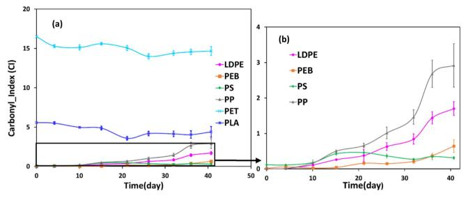
Fig. 4 (a) Temporal change in carbonyl index during accelerated weathering for different polymer samples. Carbonyl index values are expressed as average quantities  $\pm$  standard deviations of three different subsamples for each sample (n = 3). (b) Magnifies the carbonyl index for selected polymers
