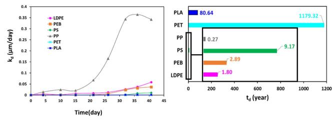
Fig. 5 Temporal changes in specific surface degradation rate (SSDR or  $k_{dr}$ , left) and the time required for total degradation ( $t_{dr}$ , right) for studied
