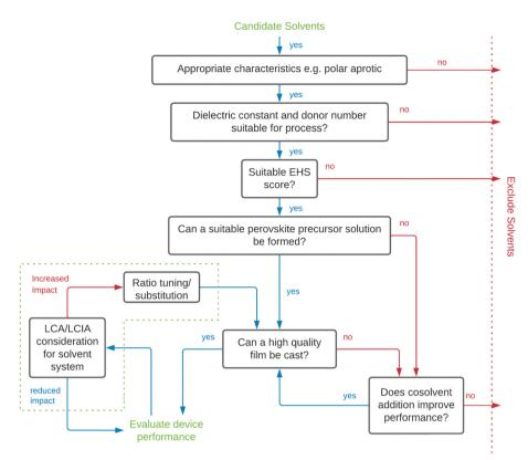
Fig. 6 Solvent selection decision tree for screening and evaluation of alternative solvents for perovskite deposition (adapted from Doolin et al.).<sup>275</sup> EHS – Environmental, health and safety, LCA - life cycle assessment, LCIA - life cycle impact assessment, MAPbl<sub>3</sub> - methylammonium lead triiodide.
