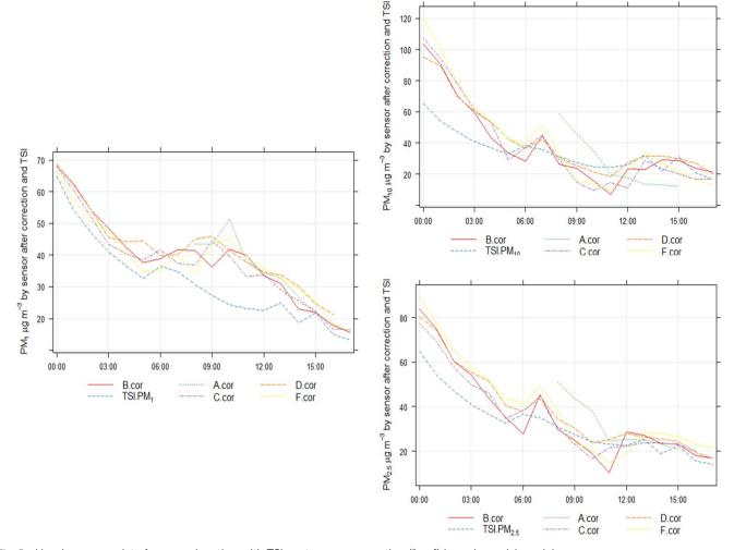
Fig. 5 Hourly average data from a colocation with TSI post sensor correction ("cor") by polynomial model.
