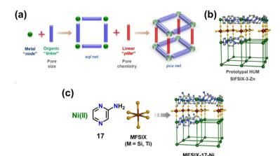
Fig. 2 (a) Schematic illustration of the modularity of pillared square grids that form the pcu topology of HUMs, (b) the prototypal pyrazine (pyz) linked HUM  $[Zn(pyz)_2(SiF_6)]_n$ , and (c) schematic illustration of the building blocks.<sup>64</sup> Reproduced with permission, Copyright 2021 John Wiley & Sons, Inc.
