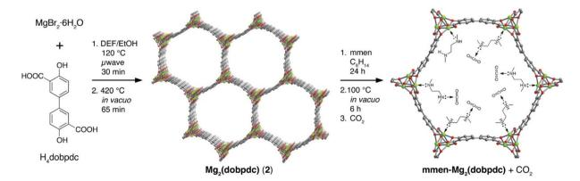
Fig. 4 (Left) Schematic of synthesis of Mg<sub>2</sub>(dobpdc) and (middle) the amine-functionalization process to produce mmen-Mg<sub>2</sub>(dobpdc), (right) interaction between pre-treated (degassed) mmen-Mg<sub>2</sub>(dobpdc) and CO<sub>2</sub> molecules. Green, red, and gray spheres represent Mg, O, and C atoms respectively; H atoms are omitted for clarity.<sup>34</sup> Reproduced with permission, Copyright 2012 American Chemical Society.
