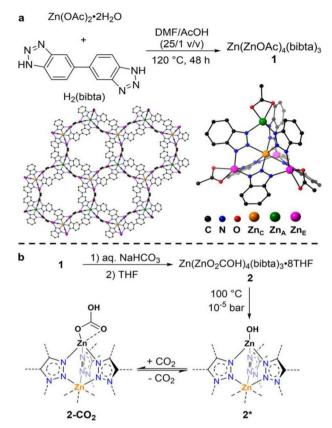
Fig. 3 (a) Synthesis structure of the Zn(ZnOAc)<sub>4</sub> SBUs. (b) Synthesis of Zn(ZnOH)<sub>4</sub>(bibta)<sub>3</sub> and mechanism of reversible CO<sub>2</sub> fixation.<sup>51</sup> Reproduced with permission, Copyright 2013 American Chemical Society.
