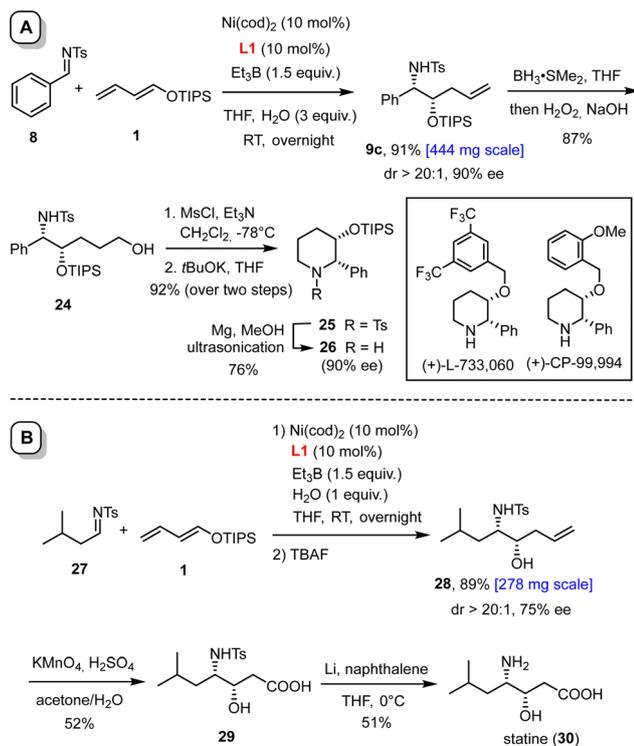
**Scheme 4** Synthetic applications. Panel A: preparation of a building block for non-peptidic neurokine NK1 receptor antagonists; panel B: synthesis of the naturally occurring  $\gamma$ -amino acid statine.
