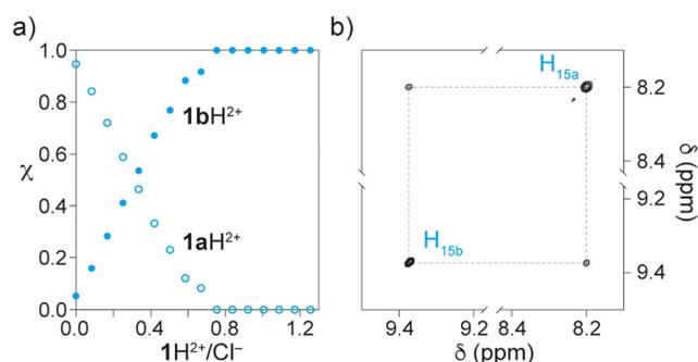
Fig. 3 (a) Titration of  $\mathbf{1aH}^{2+}\cdot 2\text{PF}_6^-$  with  $\text{tBu}_4\text{NCl}$ . Molar fraction of  $\mathbf{1aH}^{2+}$  (hollow circles) and  $\mathbf{1bH}^{2+}$  (full circles). (b) Partial EXSY spectrum (500 MHz,  $\text{CD}_2\text{Cl}_2$ , 298 K,  $t_{\text{mix}} = 200 \text{ ms}$ ) showing the chemical exchange between the triazolium signals of  $\mathbf{1aH}^{2+}$  ( $\text{H}_{15\text{a}}$ ) and  $\mathbf{1bH}^{2+}$  ( $\text{H}_{15\text{b}}$ ).
