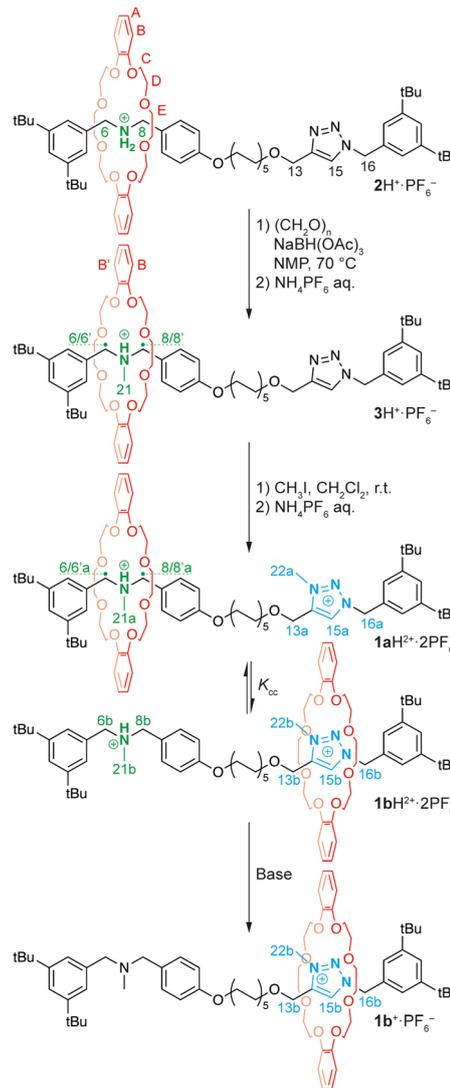
**Scheme 1** Synthesis and coconformational equilibrium of rotaxane **1aH<sup>2+</sup>·2PF<sub>6</sub><sup>-</sup>** and **1bH<sup>2+</sup>·2PF<sub>6</sub><sup>-</sup>**.
