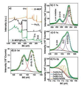
Fig. 3 (a) Survey spectra of Zr-MOF, Fe<sub>3</sub>O<sub>4</sub>, and Zr-MOF@Fe<sub>3</sub>O<sub>4</sub>; high-resolution spectra of (b) C 1s; (c) O 1s; (d) Zr 3d; (e) Fe 2p for Zr-MOF@Fe3O4
