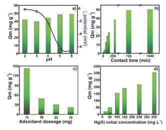
Fig. 4 Effect of (a) pH; (b) contact time; (c) adsorbent dosage; (d) Hg( $_{\rm II}$ ) concentration on the adsorption capacity of Zr-MOF@Fe $_{\rm 3}$ O $_{\rm 4}$ . Conditions: mass of Zr-MOF@Fe $_{\rm 3}$ O $_{\rm 4}$  = 30 mg, [Hg( $_{\rm II}$ )] = 50 mg L $^{-1}$ , volume = 30 mL, time = 12 h (change accordingly).
