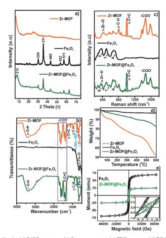
Fig. 2 (a) PXRD patterns; (b) Raman spectra; (c) FTIR spectra; (d) TGA profiles; (e) VSM curves of Zr-MOF,  $Fe_3O_4$ , and  $Zr-MOF@Fe_3O_4$ .
