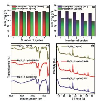
Fig. 8 Regeneration and reusability tests of Zr-MOF@Fe $_3$ O $_4$  for the removal of Hg(II) with (a) NaOH eluent and (b) HCl eluent; (c) FTIR spectra; (d) PXRD patterns of Zr-MOF@Fe $_3$ O $_4$  after reusability tests. Conditions: mass of Zr-MOF@Fe $_3$ O $_4$  = 30 mg, [Hg(II)] = 50 mg L $^{-1}$ , [NaOH]/[HCl] = 0.1 mol L $^{-1}$ , volume = 30 mL, time = 12 h.
