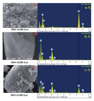
Fig. 1 SEM micrographs and EDAX analysis of (a)  $Fe_3O_4$ ; (b) Zr-MOF; (c) Zr-MOF@ $Fe_3O_4$ .
