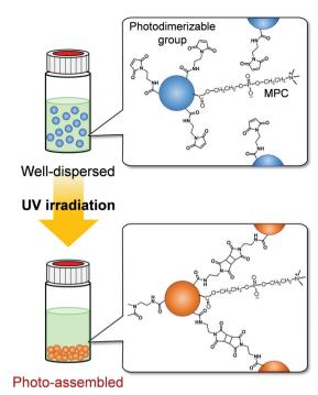
Fig. 1 Schematic representation of the photo-assembling behaviour of zwitterionic polymer particles with photodimerizable groups on their surfaces
