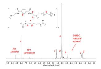
Fig. 2 <sup>1</sup>H NMR of the 1BHETA: 2PEG polyurethane in d<sub>6</sub>-DMSO.
