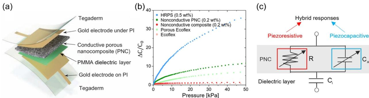
Fig. 1 (a) A schematic showing the layers of the HRPS.<sup>24</sup> (b) The HRPS is much more sensitive than the conventional CPS.<sup>24</sup> (c) A simplified circuit model to represent the hybrid piezoresistive and piezocapacitive responses of the HRPS. (a and b) Reproduced from ref. 24 with the permission of Wiley.
