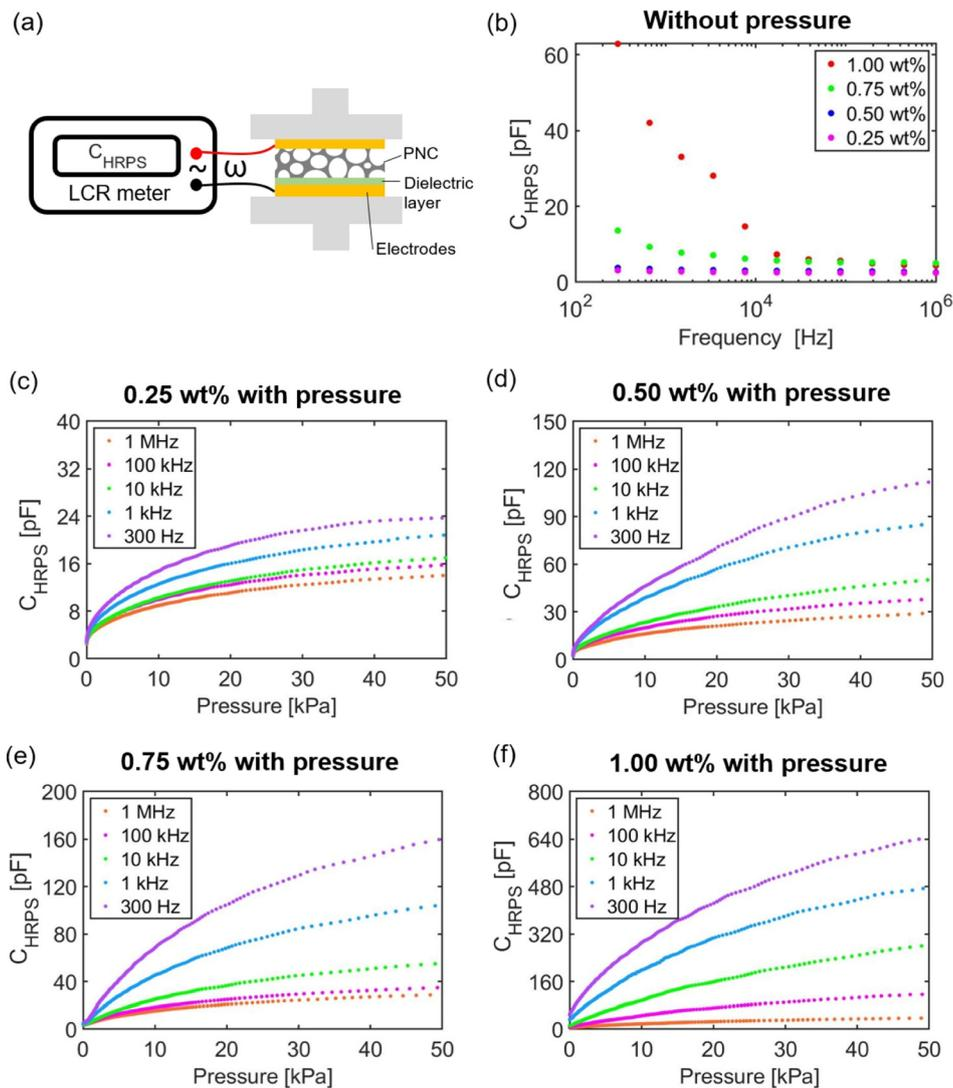
**Fig. 2** (a) A schematic of the experimental setup for measuring the HRPS capacitance without and with applied pressure at different AC frequencies. (b) Frequency response of the HRPS with different CNT doping ratios without any applied pressure. (c–f) Pressure response of the HRPS under different AC frequencies (1 MHz, 100 kHz, 10 kHz, 1 kHz, and 300 Hz) with different CNT doping ratios: (c) 0.25 wt%, (d) 0.50 wt%, (e) 0.75 wt%, and (f) 1.00 wt%.
