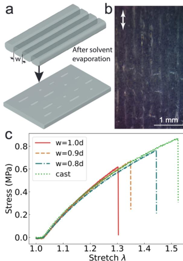
Fig. 4 (a) Schematic illustrating the relationship between the interfilament spacing,  $w$ , and the spatial distribution of defects caused by solvent evaporation after extrusion. (b) Microscope image of the surface of a sample with the printing direction indicated by the arrow. (c) Effect of the center-to-center distance between adjacent filaments, where  $d$  is the diameter of the nozzle, on the fracture response of PDUO.
