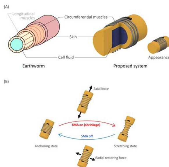
**Fig. 1** (A) Conceptual image of the single segment of an artificial hydrostat. This system has a similar configuration to the earthworm. (B) Deformation of the segment: the body is squeezed by the contraction of the SMA actuator. This causes the body to extend in the axial direction.
