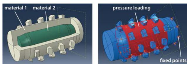
Fig. 5 The setup of the FEM model.
