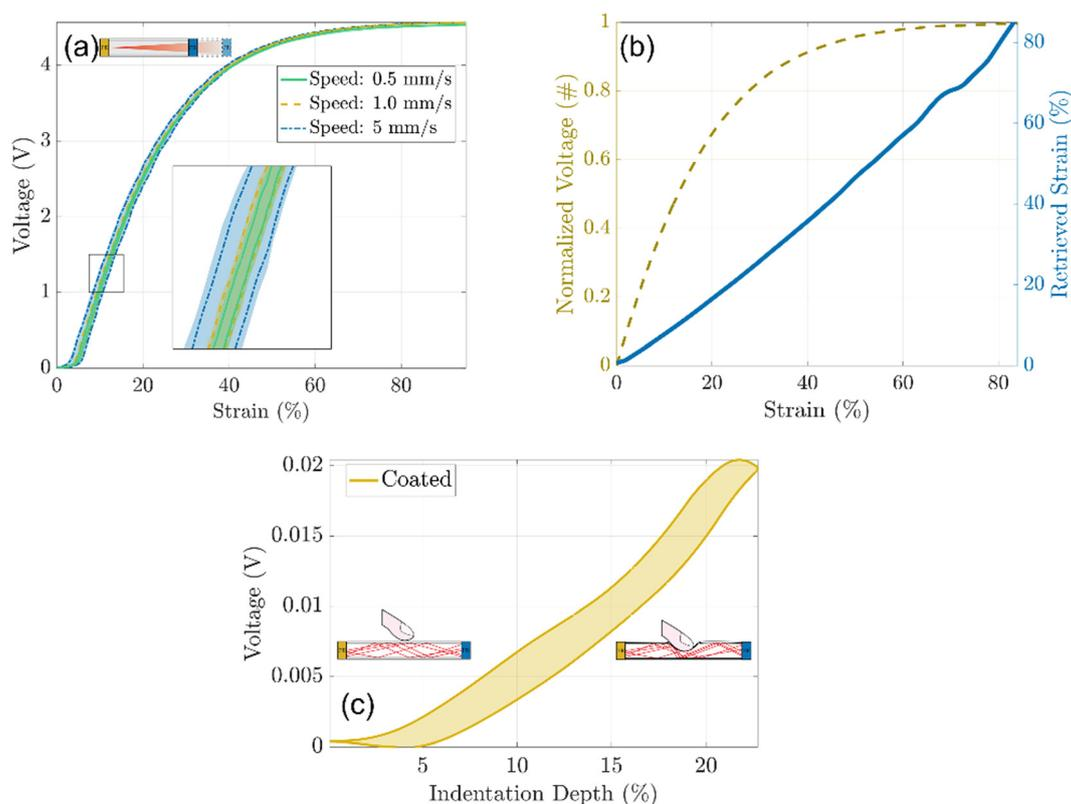
Fig. 7 (a) Voltage vs. strain% cycles of the optical strain sensor at increasing strain rate: 0.5, 1, and  $5 \text{ mm s}^{-1}$ . (b) Normalized and linearized characteristic curve of the optical strain sensor. (c) Variation in the voltage of the strain sensor when subjected to indentation. The filled portions of the curves represent the standard deviation of the measurements.
