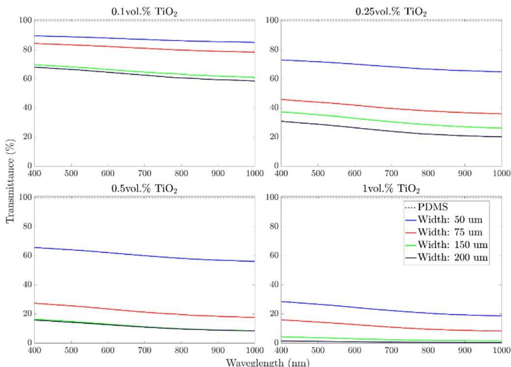
Fig. 2 UV-Vis-NIR spectrometry for 50 μm, 75 μm, 150 μm, and 200 μm thick films of PDMS\_0.1TiO<sub>2</sub>, PDMS\_0.25TiO<sub>2</sub>, PDMS\_0.5TiO<sub>2</sub>, PDMS\_1.0TiO<sub>2</sub> samples. The grey dashed line is relative to the reference sample of pristine PDMS.
