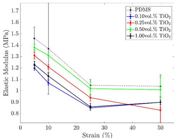
Fig. 4 Elastic module versus strain percentage of dog bone PDMS-based specimens at increasing TiO<sub>2</sub> particle concentrations. Data are acquired by uniaxial testing.
