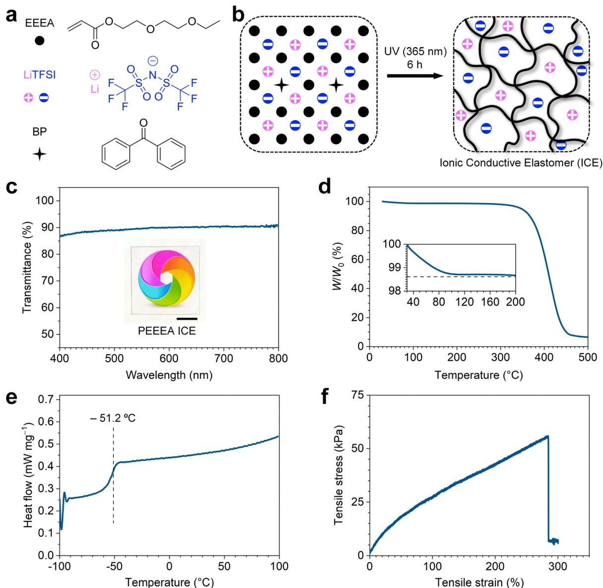
**Fig. 1** Design and physical properties of the ionic conductive elastomer (ICE). Schematics illustrate (a) the molecular structures of EEEA, LiTFSI, and BP, and (b) the synthesis of ICE. (c) Transmittance spectra of the ICE. Inset photo showing the transparency of the material. Scale bar, 1 cm. (d) TGA curve, (e) DSC curve, and (f) tensile stress–strain curve of the ICE.
