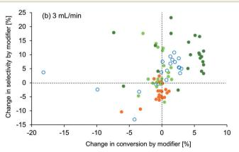
Fig. 5 Effect of 21 modifiers in terms of alkyne conversion and alkene selectivity for (a) 6 mL min<sup>-1</sup>, and (b) 3 mL min<sup>-1</sup> of total liquid flow rate. Dashed lines are displayed to show the reference value without any modifiers. Dotted lines are displayed to show the general tendency for the 6 mL min<sup>-1</sup> case.
