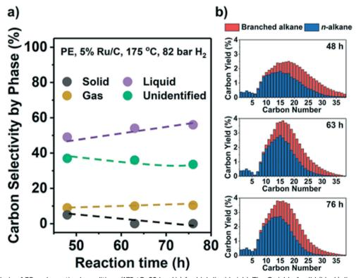
Fig. 5 Hydrogenolysis of PE under optimal conditions (175 °C, 82 bar H<sub>2</sub>) for high liquid yield. The C yield of solid (black), liquid (purple), and gas (yellow), along with unidentified C (green), are shown in a). The C distribution in  $C_1$ - $C_{38}$  products is presented in b), with gas products plotted at a one-fifth scale. A liquid yield of >57% was achieved.
