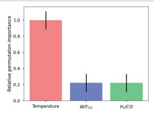
Fig. 9 Relative importance of each input feature on a global level (i.e. averaged over the entire range of operating conditions in the training dataset). The relative importance is obtained by scaling the results with that of temperature. The relative importance is calculated using the Python package, Eli5.48
