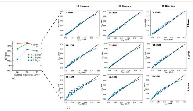
Fig. 6 R<sup>2</sup> value (a) and parity diagrams (b) of methane yield obtained with SEMK simulations and ANN predictions when using the validation dataset. Different ANN models with 1-3 hidden layers and 10-30 neurons in each layer are shown.
