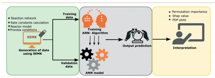
Fig. 3 Schematic representation of the different steps involved in ANN model development and interpretation of the model. Data from SEMK simulations (green box) are used for training the ANN model (grey box) which is then analysed using different interpretation techniques (yellow box).
