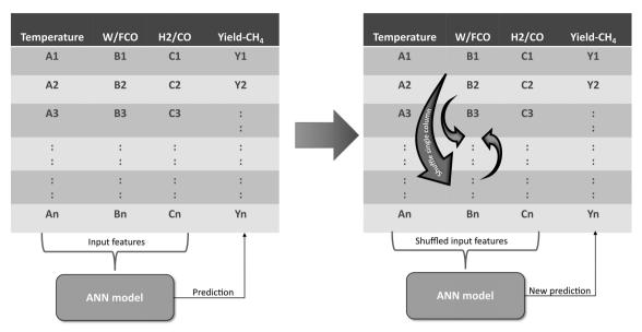
Fig. 4 Graphical representation of the permutation importance principle. The model error is calculated using the ANN prediction without permutation (left) and the ANN prediction with permutation (right) of input features such as W/F<sub>CO</sub>.
