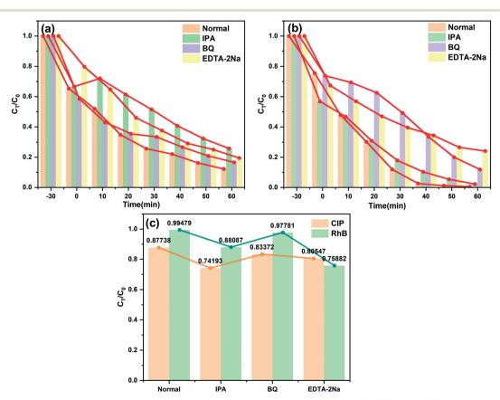
Fig. 13 The radical quenching results of the NMFA-5 composite for the degradation process of the CIP (a) and RhB (b), and the results comparison (c).
