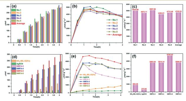
Fig. 11 The H<sub>2</sub> evolution performances of the NMFA-5 composites for five cycles (a)-(c), and different samples (d)-(f) under the same reaction conditions.
