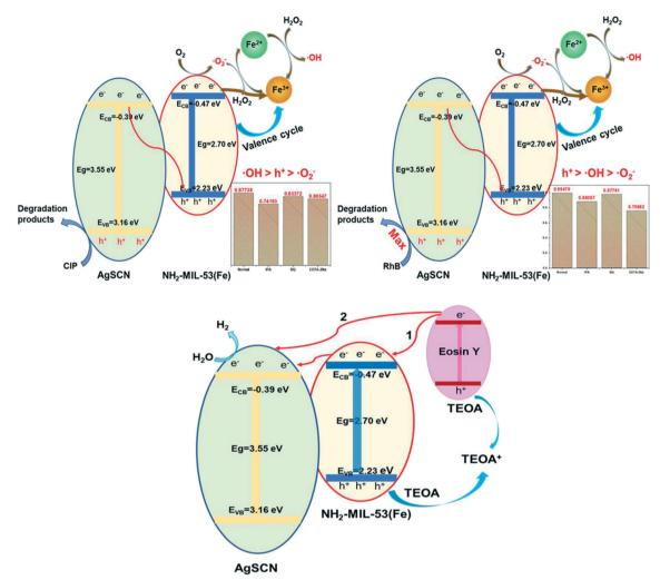
Fig. 15 Proposed schematic diagram of the possible charge transfer approach of the NMFA composite for the degradation of pollutants and hydrogen production.
