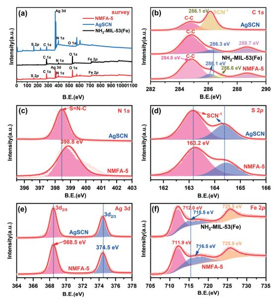
Fig. 5 XPS spectra of (a) the survey scan, and (b) C 1s, (c) N 1s, (d) S 2p, (e) Ag 3d, and (f) Fe 2p for the samples.
