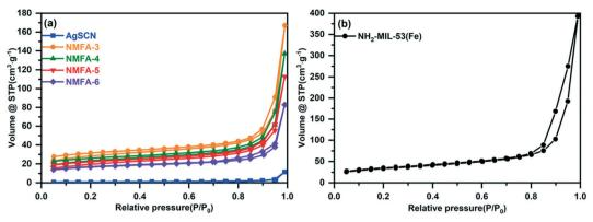
Fig. 7 The N<sub>2</sub> adsorption-desorption isotherms for the (a) AgSCN and NMFA-x, (b) NH<sub>2</sub>-MIL-53(Fe).
