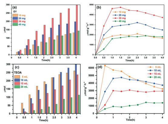
Fig. 10 The effect of the photosensitizer EY (a) and (b) and TEOA (c) and (d) on the H<sub>2</sub> production performance.
