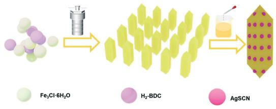
Fig. 1 Schematic illustration of the process for preparing the NH<sub>2</sub>-MIL-53(Fe)/AgSCN composites.
