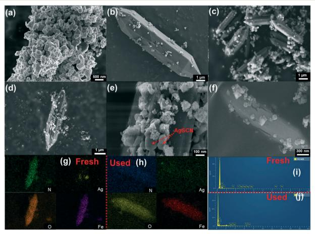
Fig. 2 SEM images of (a) AgSCN, (b) NH<sub>2</sub>-MIL-53(Fe), (c)-(e) NMFA-5 and (f) NMFA-5 after H<sub>2</sub> production, element mapping results (g) and (h), and EDX spectra (i) and (j) of fresh NMFA-5 and after H<sub>2</sub> production.
