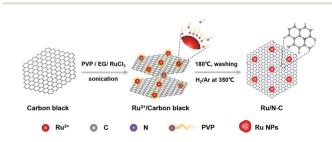
Fig. 1 Schematic diagram of the synthesis of Ru/N-C.
