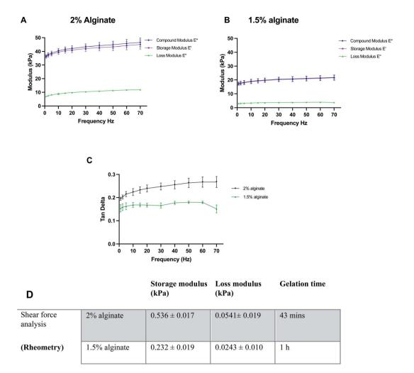
Fig. 2 Characterisation of the mechanical properties of different alginate formulations: compressive dynamic mechanical properties of different concentrations of alginate; (A) 2% alginate, (B) 1.5% alginate and (C) tan delta for both conditions. (D) Overview of rheological properties of alginate specimens. Data expressed as means  $\pm$  SD, N=3.
