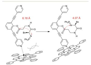
Fig. 3 Schematic representation of calculated structures of cisoid isomers of iminophosphorane intermediates 3 and (Turbomole, BP86, def2-TZVP) with N-C distances in red.
